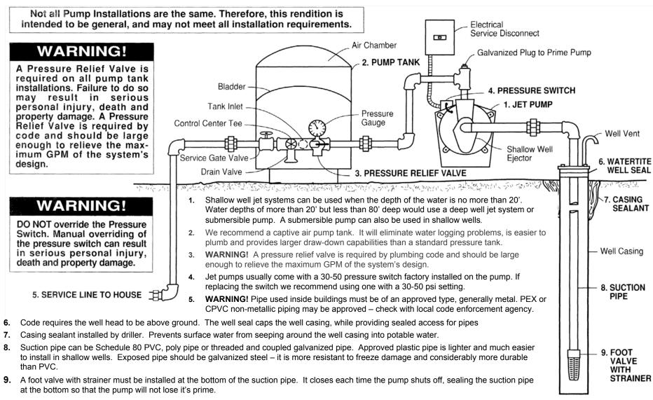
**IMPORTANT!** When the pump is first started, it should be left running until test samples clear up and are completely free of sand.
