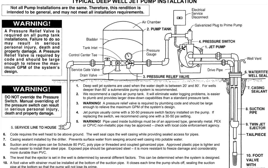
IMPORTANT! When the pump is first started, it should be left running until test samples clear up and are completely free from sand.
